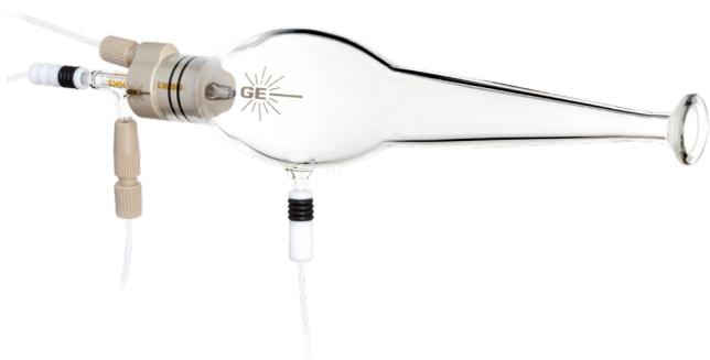
Conventional ICP-MS spray chambers have low transport efficiencies (< 5%) and filter out larger droplets (>5µm) preventing a high percentage of cells from entering the plasma. As most cell lines of interest are larger than 5µm, the spray chamber design for single cell analysis is different from conventional ICP-MS spray chambers.
