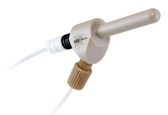
Samples with residual hydrofluoric acid (HF) require an inert nebulizer made of PEEK, PFA or alumina - glass or quartz nebulizers are not suitable for these sample matrices.
