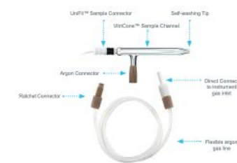
Figure 1. Details of SeaSpray DC nebulizer (PIN A31-07-J852)
