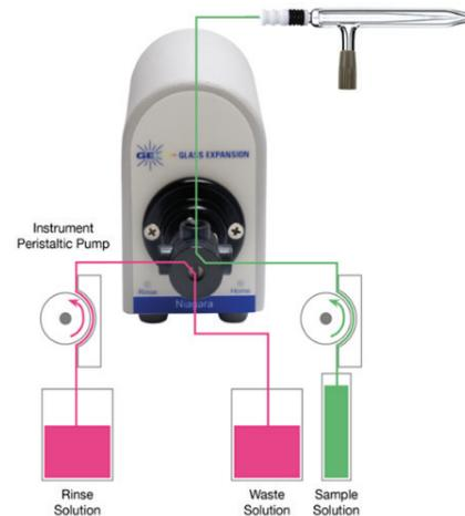
**Figure 1b.** Rinse to nebulizer; sample to waste (rinse position)
