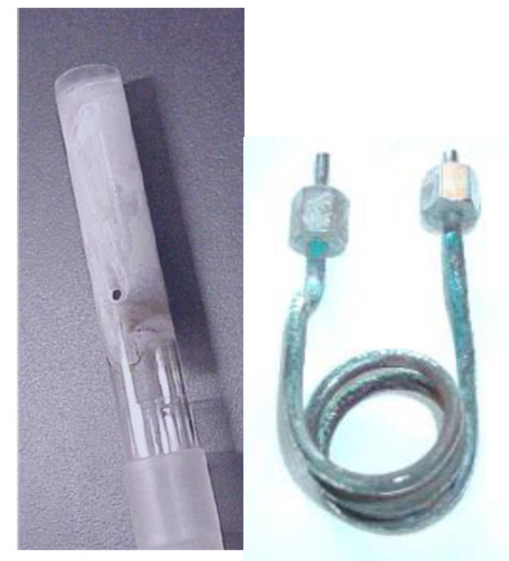
Devitrification of quartz due to salt deposits (Left), and RF Coil corrosion (Right)
