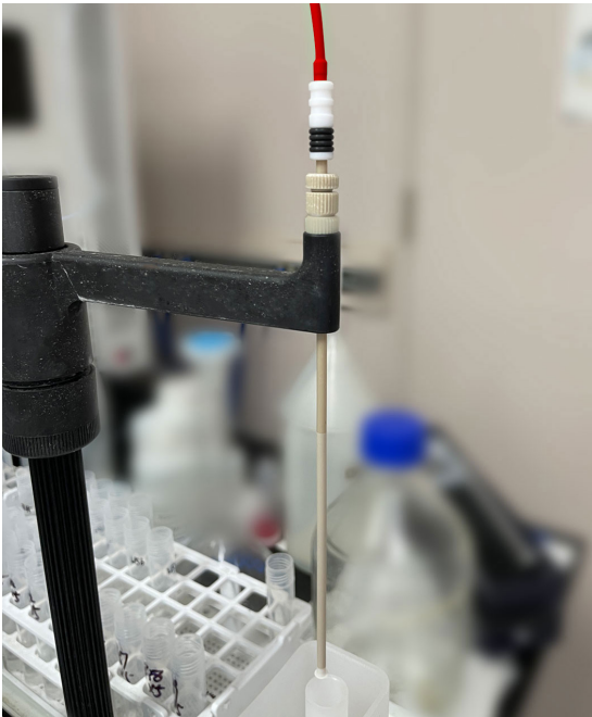
P/N 70-803-2953 installed on ESI® SC-DX Autosampler
