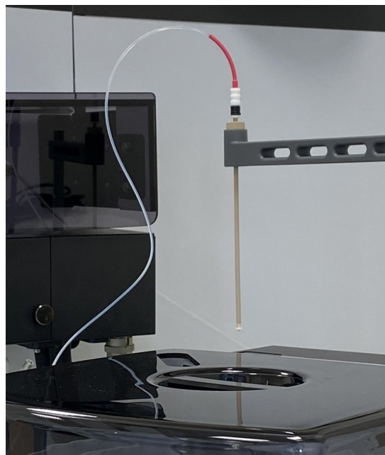
P/N 70-803-2872 installed on Shimadzu® AS-20 Autosampler
