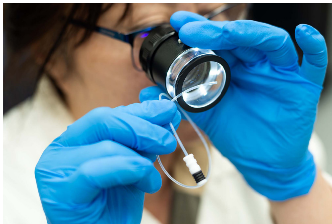
Check condition of Capillary Tubing
