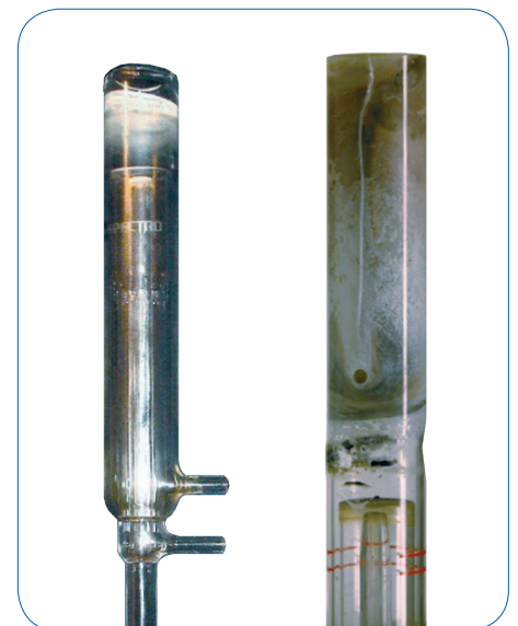
Figure 3: Examples of devitrification of quartz torches
