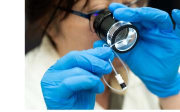
**Check condition of Capillary Tubing**
