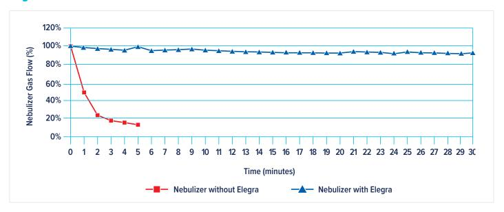
The graph above is the result of an extreme test, aspirating a 25% salt solution continuously without rinsing. Without the Elegra, the nebulizer begins to clog after only a few minutes as designated by the steep decrease in nebulizer flow. However, with the Elegra installed, the nebulizer is stable for well over 30 minutes.
